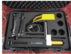
Flange hole alignment jig
